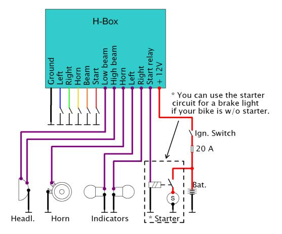
**Push button or switch input for the left flashers (blue):** You can use this input for a push button or a switch what will connect the input to ground / chassis when pressed. An close contact will start the flasher left.
